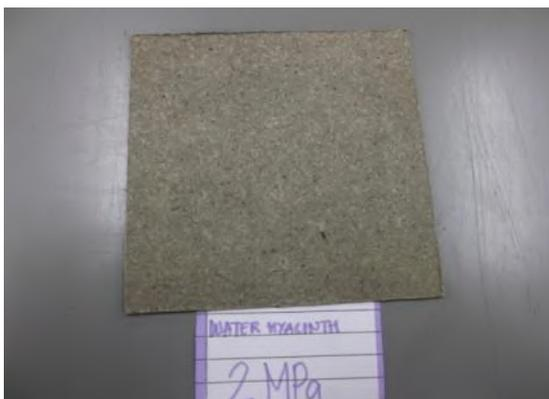
Fig 2. Water hyacinth bio-board successfully produce
